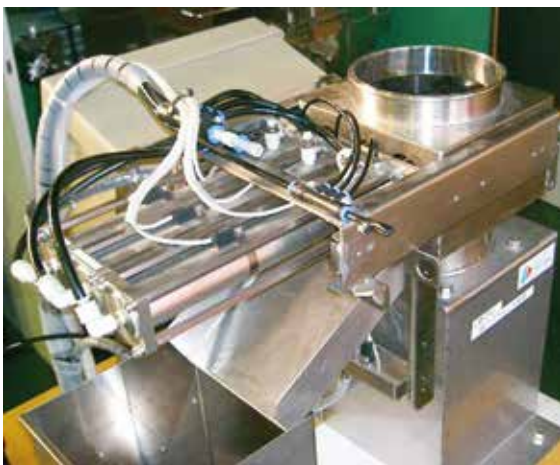
Auto-cleaning model (all metal powder cleaning process is automated by actuator)
