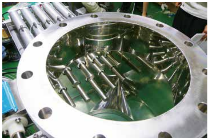
Auto-cleaning model (all metal powder cleaning process is automated by actuator)
